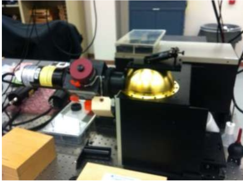
Figure 2.6.5. Gooch and Housego OL Series 750 Spectroradiometric Measurement System with an OL 740-70 integrating sphere reflectance attachment.
