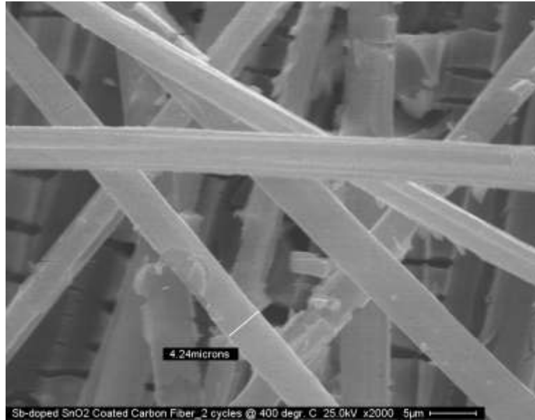
Figure 5.3.3. ATO coated carbon fibers heat treated at 400 °C.
